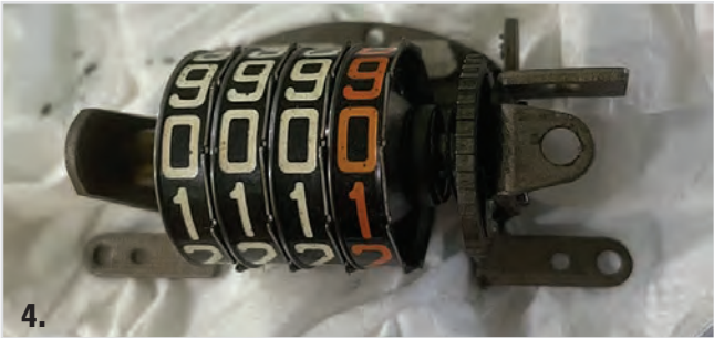
Trip Odometer disassembly to change toothed wheel
