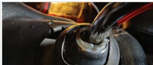
Damaged plastic dome washer.
