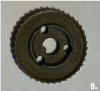
Trip Odometer disassembly to change toothed wheel
