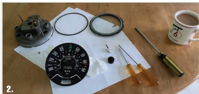
Speedometer disassembly – Note toothed wheel tooth count labelled
