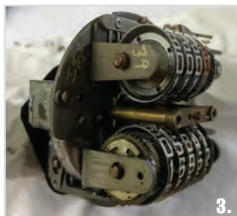
Speedometer disassembly – Note toothed wheel tooth count labelled
